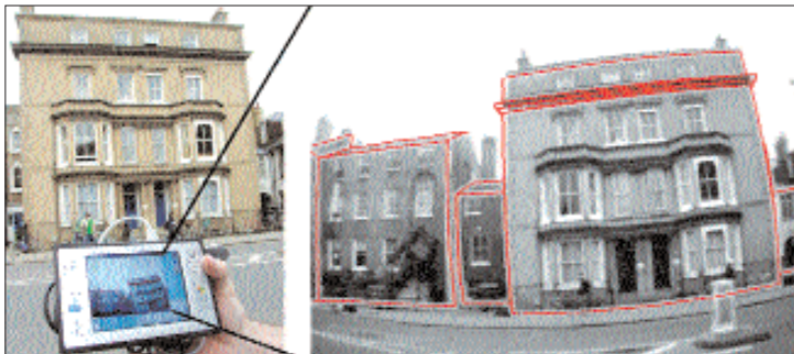
Just one aspect of the AR problem. User points AR device at object; device collates lots of measurements; edges are detected. Even this is hard!
